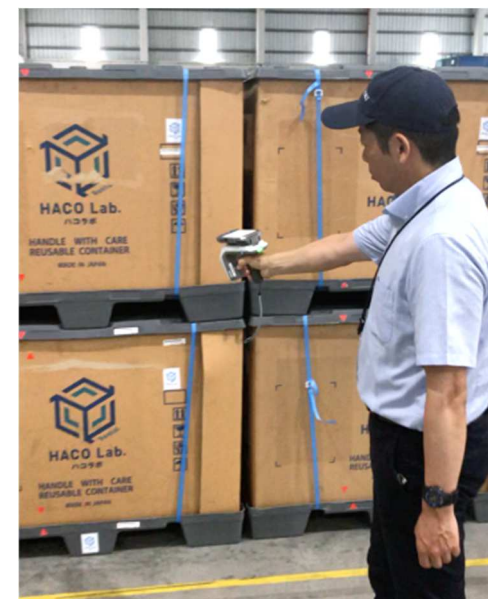
Checking numbers of pieces in each pallet box all at once by scanning the RFID tags
